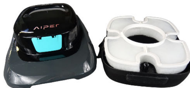
Fig. 1 Cleaner opened with filter grid
